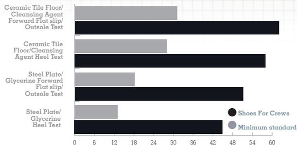
Slip Resistance Test EN ISO 13287:2012, performed by TÜV Rheinland LGA Products GmbH in Leipzig, Germany during August 2018\* On a scale where 0.0 is the absence of friction and 1.0 is very high friction (e.g. dry carpet), SFC rated .63 - more than tripling the .18 minimum standard. All SFC shoes use the Shoes For Crews patented slip-resistant outsole. Product tested: BRIDGETOWN 28740
